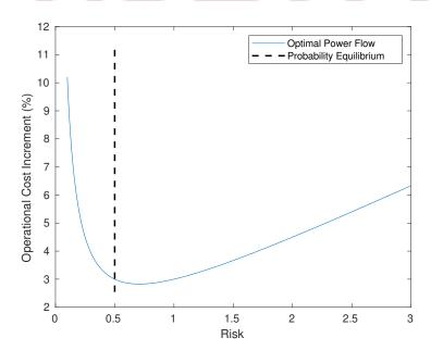
Figure 7: Optimal Power Flow at Different Level of Risks
